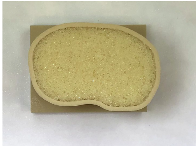
Figure 2. The Sawbone® models, (Pacific Research Laboratories Inc. Vashon, WA, USA) were made using firm polyurethane foam. The density of the foam is 12.5 lb per cubic foot (PCF) for simulating cancellous bone and 40 PCF for simulating the outer cortical shell (product reference: 1522-912). As per the manufacturer, both materials comply with the ASTM F1839-08 material standard. The model has a rectangular base of approximately 5.7 cm in width, 7.6 cm in length, and 7.6 cm in height. The proximal end has been shaped to correspond to the tibia, measuring 46.2 × 75.3 mm.
