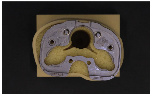
Figure 3. Top view of the prepared bone model showing the surgical guide used during the process, the drilled stem hole and the broach for the cruciate stem.
