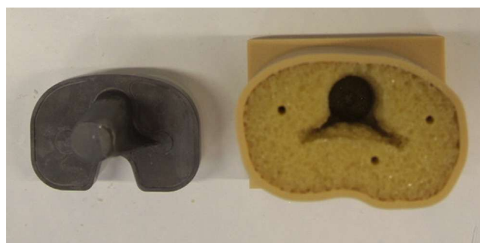
Figure 1. NexGen Stemmed Option size 4 tibial plateau (left). Tibia Plateau Block, Cellular Core 12.5 PCF with Solid Foam Shell 40 PCF after preparation (right).
