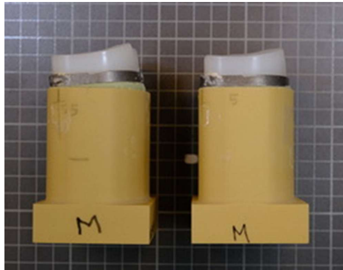
Figure 7. Photography of FC (left) and SC (right). Note difference in cement mantle thickness anterior to posterior and baseplate posterior tilt on FC.
